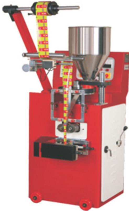
Use For : This Form Fill / Seal / Machine Is Use To Pack Paste, Cream, Cosmetic Paste, 'C' Oil, Etc... Semi Liquid Products
